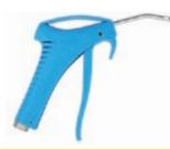
Fluids: compressed air Materials: technical polymer, NBR Pressure: 10 bar Temperature: -15°C to +50°C (DN): 3.5 mm
